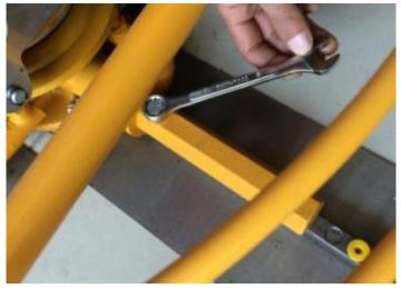
4. Loosen the outside bolt with the 1/2 in. wrench (Fig. 3).
