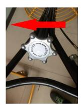
4. Continue to turn the Blade Pitch Handle counter-clockwise until the Adjust Screw Nut is at the bottom.
