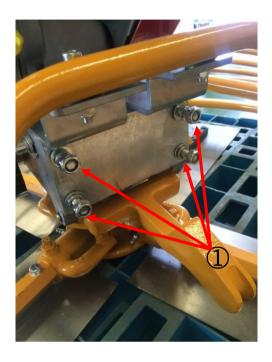
2. Tighten the Nuts with the 17mm wrench. Torque should be 60 ft-lbs. (830 kgf.cm).
