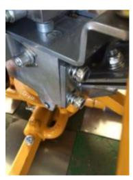
3. Turn the Blade Pitch Handle counter-clockwise.
