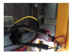
12. Remove a bolt from the engine housing, put the ring terminal of the Engine Stop Switch over the bolt, replace the bolt and retighten it.
